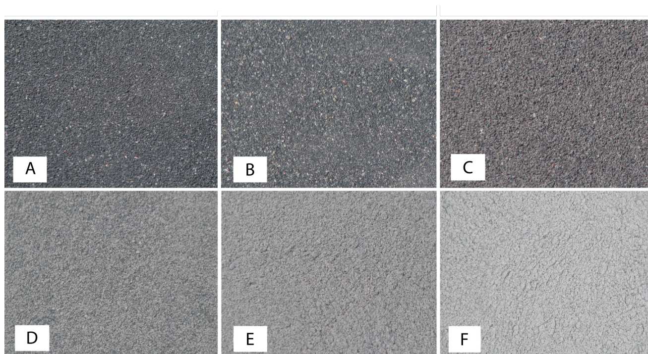
Figure 4: Photographs of six tephra materials erupted by Tungurahua volcano, each being characterised by different <63\ \mu\text{m} -particle contents: <5\% [A]; 5 \leq x < 10\% [B]; 10 \leq x < 20\% [C]; 20 \leq x < 30\% [D]; 30 \leq x < 40\% [E]; and \leq 40\% [F].
