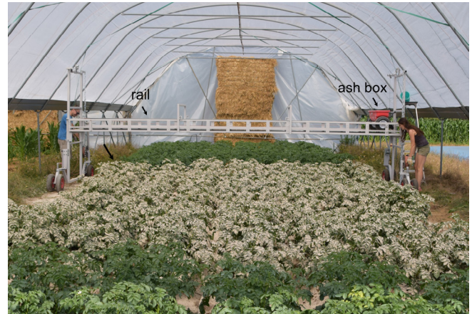
Figure 2: Photo of the ash spreader used to apply ash to the crop plants (here potatoes). The ash spreader consists of an ash box installed on a 7-m-long rail. The spreader is pulled manually with a rope allowing ash particles to exit the device through 20 holes located at the bottom of the ash box.
