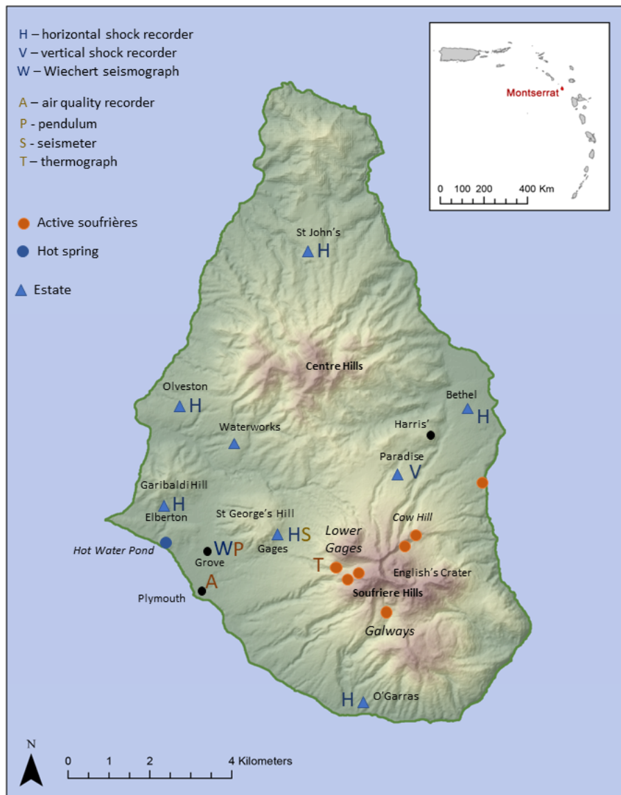
Figure 5: Map showing locations of instruments deployed by Perret in 1934–45 (pendulum, seismeter, thermograph) and 1937 (air quality recorder) and Powell or the staff of the seismo-volcanic observatory in 1936 (horizontal shock recorders, H; vertical shock recorder, V and Wiechert 2-component seismograph).
