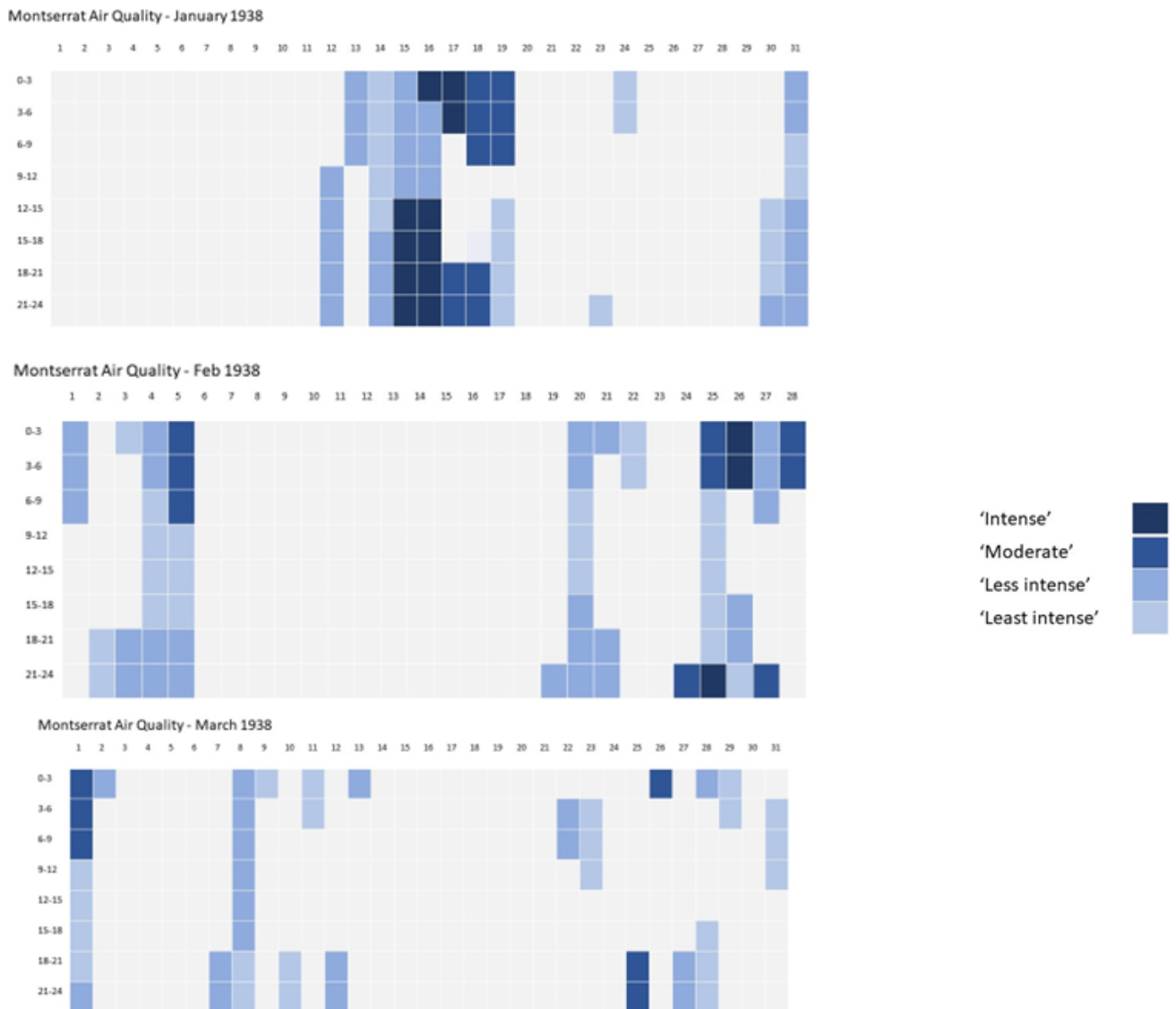
Figure 9: Summary of qualitative air quality measurements in Plymouth, January–March 1938 recorded in the monthly reports of the seismo-volcanological observatory. Boxes are coloured according to the reported intensity, the x-axis represents the day of the month, the y-axis the time. The intensity of discolouration of the disc was assessed by the observer using a simple relative intensity scale. Moderate to intense discolouration corresponded to times when the smell of \text{H}_2\text{S} in Plymouth was ‘strong’ or ‘unpleasant’; and many of the most noticeable episodes were late evening or early morning. Less intense discolouration corresponded to episodes when the smell of \text{H}_2\text{S} was weak to barely noticeable. During windy weather, there was often no discolouration of the discs.
