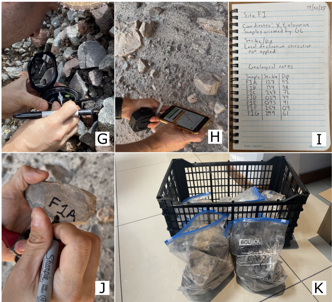
Figure 8: (Continued from previous page) [G] measuring the strike of the sample with the geological compass, [H] measuring the strike and dip of the flat sample face with a smartphone compass-clinometer app, [I] example of a standard field notebook table with sample names and orientations, [J] oriented sample being labeled with its sample name after removal from the outcrop, [K] samples from a single site organized together in a well-labeled sample bag.
