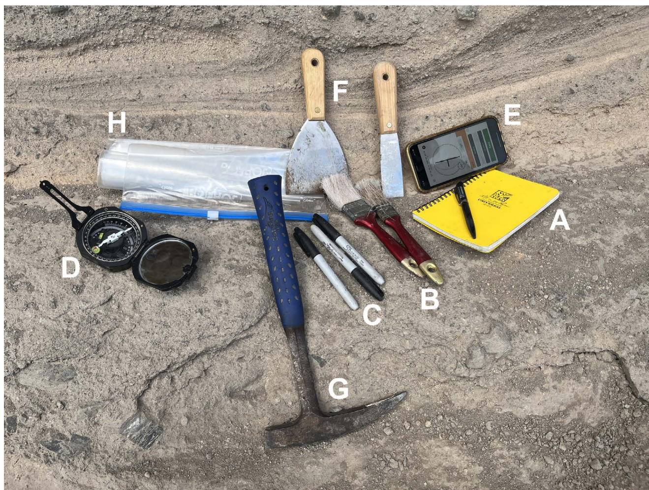
Figure 7: Key equipment for paleomagnetic sampling of pyroclastic deposits: [A] Field notebook, [B] brushes of varying sizes for cleaning rock samples before labeling, [C] permanent markers for labeling, [D] example of a geological compass-clinometer for orienting samples, [E] example of a smartphone compass-clinometer app that can also be used for sample orientation, [F] metal spatulas of varying sizes for cleaning the outcrop and the samples, [G] geological hammer/pick for cleaning the area around the sample and removing the sample from the outcrop, [H] cloth and plastic sample bags for organizing oriented samples.
