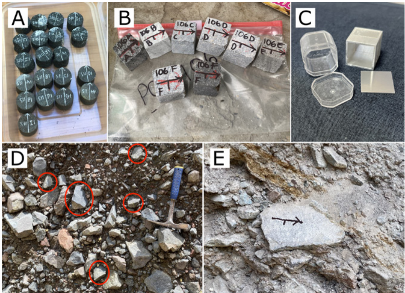
Figure 6: Photos showing important paleomagnetic sample and specimen characteristics. [A] example of 25 mm diameter, 25 mm-long cylindrical rock specimens, [B] 2 \times 2 \times 2 cm rock cube specimens, [C] specialized plastic and metal boxes for collecting 2 \times 2 \times 2 cm cubic samples of ash matrix, [D] PDC outcrop with several viable hand samples highlighted, [E] example of an ideal hand sample, note the flat face of rock that is ideal for measuring and labeling.
